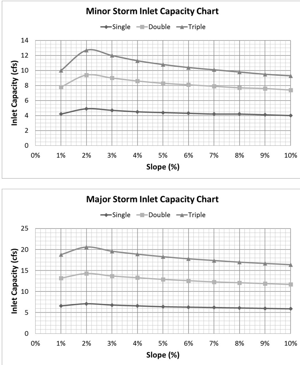
**Figure 8-2. Inlet Capacity Chart, Minor Residential (Local) Streets Inlets on Grade
