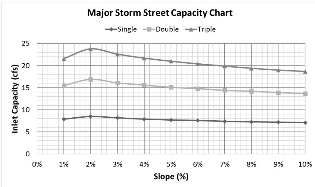
**Figure 8-1. Inlet Capacity Chart, Residential (Local) Streets Inlets on Grade
